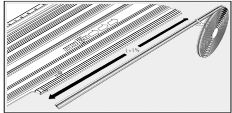
Fig. 12: Inserting the new chip breaker guard
