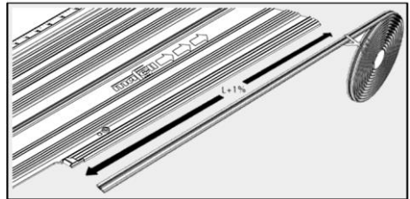
Fig. 12: Inserting the new chip breaker guard
