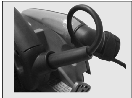
Fig. 3: Routing the connecting cable
