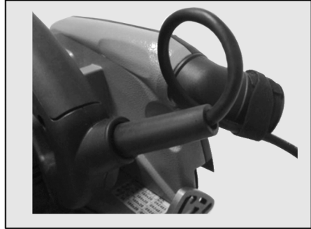
Fig. 6: Routing the connecting cable
