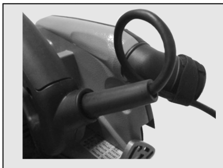
Fig. 3: Routing the connecting cable
