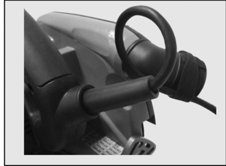
Fig. 6: Routing the connecting cable
